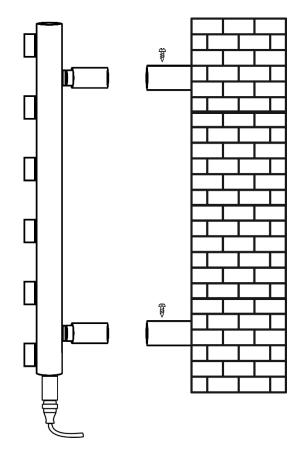
You are now ready to run, adjust and connect your piping and valve to the radiator valve tail and Tpiece inserted into the radiator during step 2.
