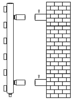
You are now ready to run, adjust and connect your piping and valve to the radiator valve tail inserted into the radiator during step 2.
