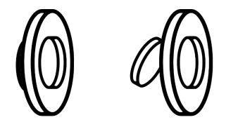
Attach rubber rings (K) (if not already applied) and apply PTFE tape to blanking plug (A) and air vent (B). Insert into top 2 threads of radiator, cover with a cloth to prevent damage to the radiator and tighten with spanner.
