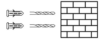
Insert the 2 screws (D) for each hook. Fully tighten the 2 screws for the top 3 hooks, and partially tighten the 2 screws for the bottom 3 hooks.
