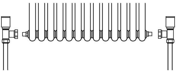
Prior to operating the radiator, you may need to flush the system to clear any residue.
