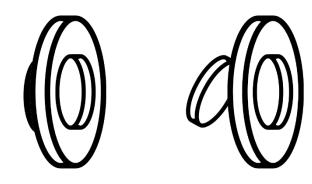
Attach rubber rings (K) (if not already applied) and apply PTFE tape to blanking plug (A) and air vent (B). Insert into top 2 threads of radiator, cover with a cloth to prevent damage to the radiator and tighten with spanner.
