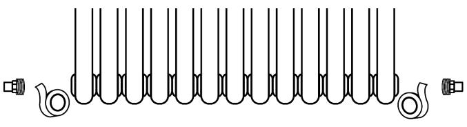
In your desired location, mark the 2 drill points for each of the 4 hooks (E) using a pencil. These should install at least 1 column from either end, the brackets go around the column.
