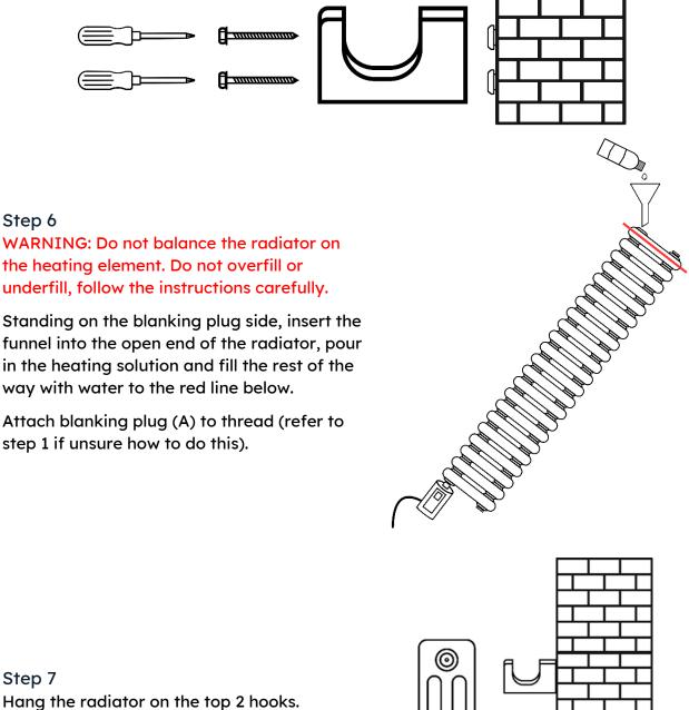
Adjust the bottom 2 hooks and fully tighten the 2 screws with a spanner.
