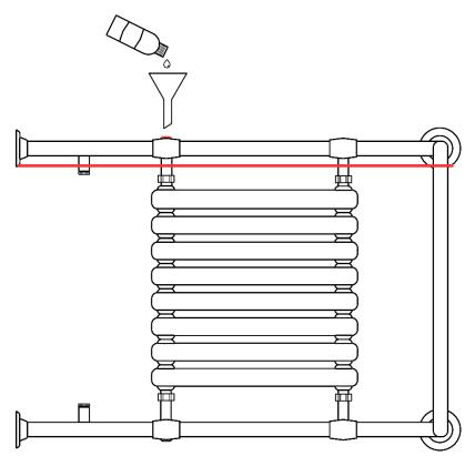
Using the electric element instructions, insert the element to the same location, being careful to manage any spillage that may occur.
