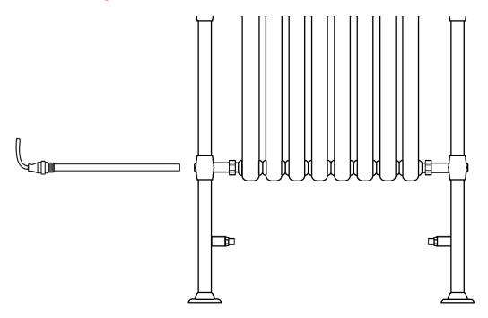
(Check valve instructions) – If appropriate, apply PTFE tape to valve tails and insert into bottom 2 threads of the radiator and tighten with a spanner.
