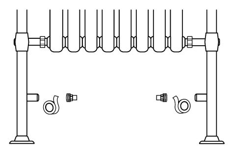
You are now ready to run, adjust and connect your piping and value to the radiator value tail inserted into the radiator during step 2.
