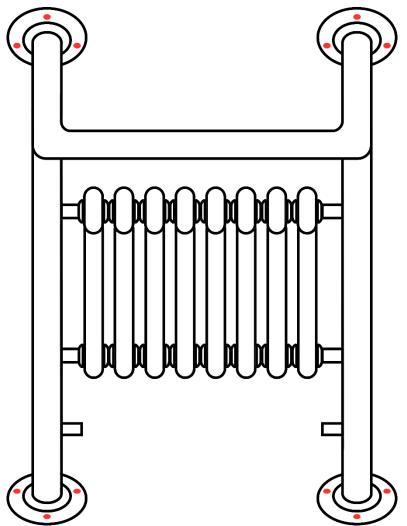
Using the drill and 8mm masonry drill bit, drill a hole in the marked locations (Note: on tiles walls you may need to use a tile drill prior to masonry).
