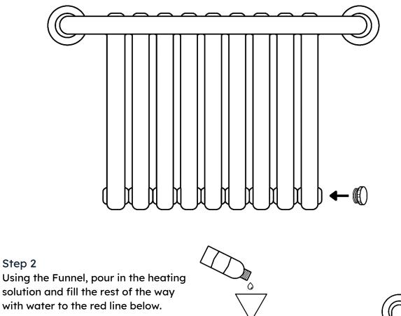
Using the electric element instructions, insert the Element to the same location, being careful to manage any spillage that may occur.
