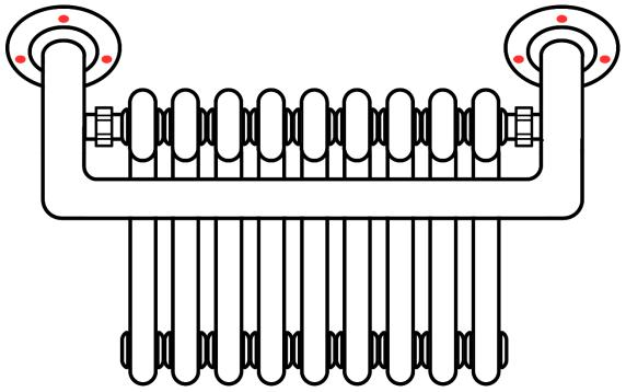
Using the drill and 8mm masonry drill bit, drill a hole in the marked locations (Note: on tiles walls you may need to use a tile drill prior to masonry).
