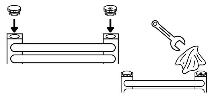
Step 2 (Check element instructions) - Apply PTFE tape to the additional blanking plug and insert on one side of the bottom of the radiator. Insert the element per the element instructions on the other side of the radiator.
