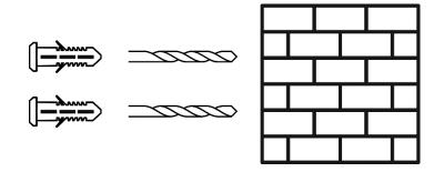
Insert the 2 screws (D) for each hook. Fully tighten the 2 screws for the top 2 hooks, and partially tighten the 2 screws for the bottom 2 hooks.
