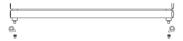
The wall supports will insert between 2 of the bars, they should be measured approximately 100mm from the vertical tube.
