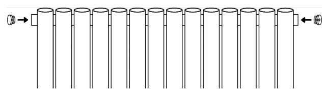
Step 3 (Check element instructions) - Using PTFE tape, insert the element per the element instructions on the other side of the radiator.
