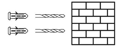
Insert the 2 screws (D) for each hook. Fully tighten the 2 screws for the top 2 hooks, and partially tighten the 2 screws for the bottom 2 hooks.
