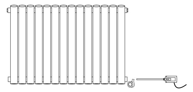
In your desired location, mark the 2 drill points for each of the 4 hooks (E) using a pencil. These should install at least 1 column from either end, the brackets go around the column.
