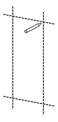
Step 5 Using the 8mm masonry drill bit, drill holes at the marked location and insert masonry wall plugs (C).
