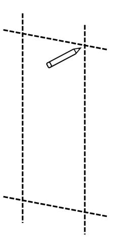
Using the 8mm masonry drill bit, drill holes at the marked location and insert masonry wall plugs (C).
