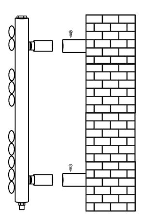
You are now ready to run, adjust and connect your piping and valve to the radiator valve tail inserted into the radiator during step 2.
