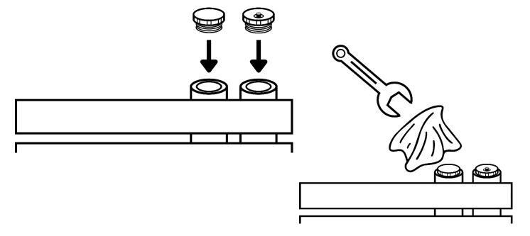
Step 2 (Check Valve Instructions) – If appropriate, apply PTFE tape to valve tails and insert into bottom 2 threads of the radiator and tighten with a spanner.
