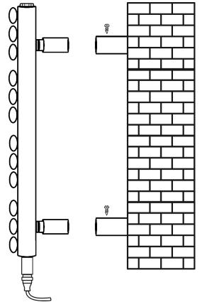
You are now ready to run, adjust and connect your piping and value to the radiator value tail and T-piece inserted into the radiator during step 2.
