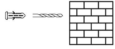
Place the long screw (D) through wall support (E) and tighten into the wall plug.
