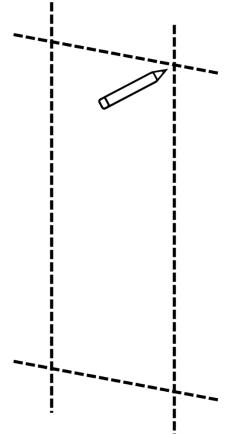
Using the 8mm masonry drill bit, drill holes at the marked location and insert masonry wall plugs (C).
