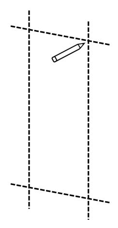
Using the 8mm masonry drill bit, drill holes at the marked location and insert masonry wall plugs (C).
