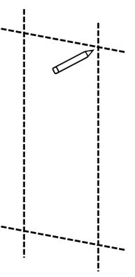
Using the 8mm masonry drill bit, drill holes at the marked location and insert masonry wall plugs (C).
