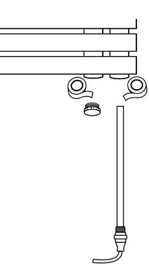
Step 3 Put bolt (H) through bracket (F) and screw onto the back of the radiator at the pre-drilled locations.
