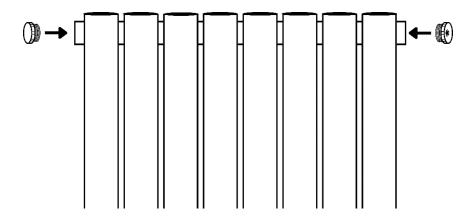
Step 2 (Check Valve Instructions) – If appropriate, apply PTFE tape to valve tails and insert into bottom 2 threads of radiator and tighten with a spanner.
