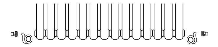
In your desired location, mark the 2 drill points for each of the 4 hooks (E) using a pencil. These should install at least 1 column from either end, the brackets go around the column.
