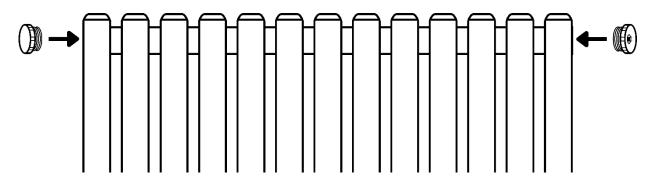
Step 2 (Check Valve Instructions) – If appropriate, apply PTFE tape to valve tails and insert into bottom 2 threads of radiator and tighten with a spanner.
