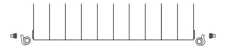
In your desired location, mark the 2 drill points for each of the 4 hooks (E) using a pencil. These should install at least 1 column from either end, the brackets go around the column.
