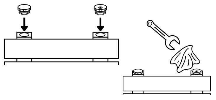
Step 2 (Check Valve Instructions) – If appropriate, apply PTFE tape to valve tails and insert into bottom 2 threads of the radiator and tighten with a spanner.
