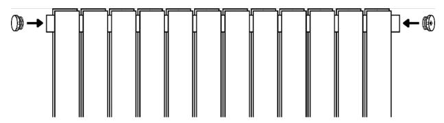
Step 3 (Check element instructions) - Using PTFE tape, insert the element per the element instructions on the other side of the radiator.
