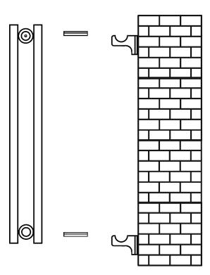
You are now ready to run, adjust and connect your piping and valve to the radiator valve tail inserted into the radiator during step 2.
