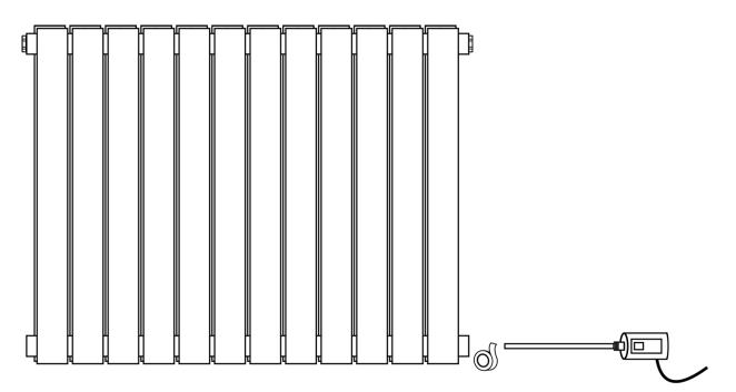
In your desired location, mark the 2 drill points for each of the 4 hooks (E) using a pencil. These should install at least 1 column from either end, the brackets go around the column.
