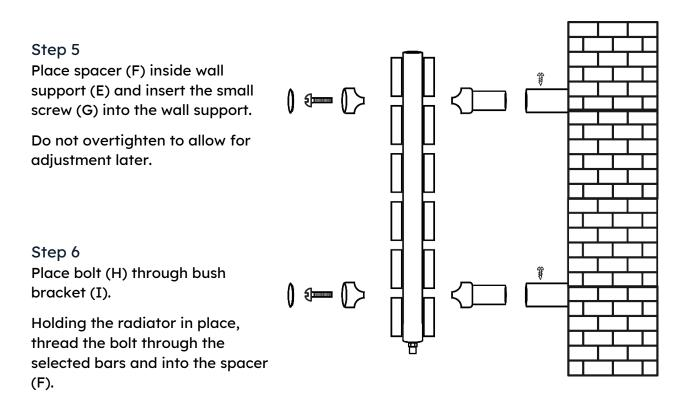
Adjust to required depth and tighten small screw (G).
