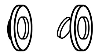
Attach rubber rings (K) (if not already applied) and apply PTFE tape to blanking plug (A) and air vent (B). Insert into top 2 threads of radiator, cover with a cloth to prevent damage to the radiator and tighten with spanner.
