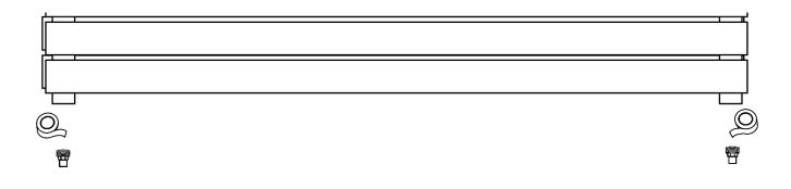
The wall supports will insert between 2 of the bars, they should be measured approximately 100mm from the vertical tube.
