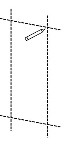
Step 5 Using the 8mm masonry drill bit, drill holes at the marked location and insert masonry wall plugs (C).
